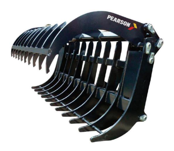
Built tough to last, Pearson Heavy Duty Grapples are made using Bisalloy – a high tensile steel with a yield strength three times greater than mild steel and excellent wear resistance. All surfaces that touch the load are fully Bisalloy armoured meaning you get a longer life from your investment. Heavy wall RHS locks the tines together creating a rigid subframe allowing the heavy duty grapple to lift uneven loads without twisting.
