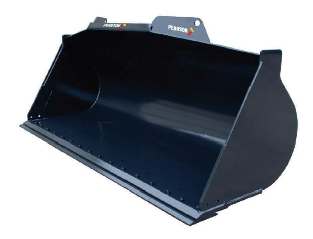
The Pearson Wheel Loader is an extra heavy duty bucket specifically designed for use with wheel loaders. It has the biggest cutting edge of our bucket range at 35mm thick and 300mm deep. These buckets come standard with a sacrificial blade that is made from hard-wearing 500HB abrasion resistant steel; this blade takes the impact and improves the life of the bucket, so you get extra value from your investment.
