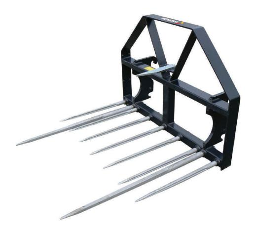
Handle big bales and silage without having to change implements in between! The Pearson Combo Fork is a popular choice for many farmers because it is built to last and saves you time. Made from thick wall RHS with hard-wearing 2 pack paint and high-quality German tines with conus 1 and 2 bushes to prevent loosening and spinning.
