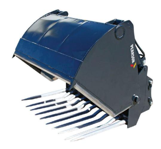
Eliminate spoilage and wastage with the Pearson Shear Grab. A highly powerful ram for clean cutting force. Additional razor sharp Bisalloy cutting knives offer optimum operational efficiency leaving a clean-cut face and minimal waste. It's easy to maintain a super sharp cutting edge while keeping oxygen out and minimising rot. This grab also provides an effective solution to moving maize without risking aeration.
