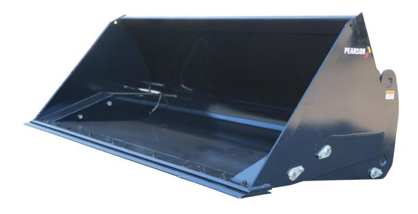
The Pearson High Tip Bucket is perfect for loading of high-sided trailers whilst keeping all the reach of a horizontal bucket. A rigid frame and powerful rams gives the bucket all the strength required for heavy lifting. 35mm pins and DX bushes ensures that this bucket is here for the long haul.
