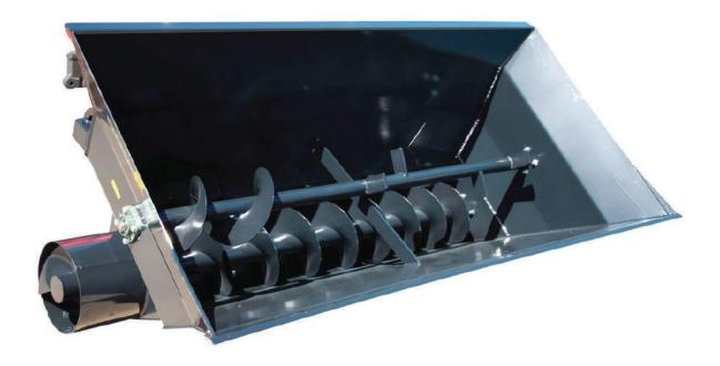
Pearson Auger Buckets are specifically designed to handle fine chop maize silage, meal mix etc. At 500kg these units are best suited to smaller tractors from 80hp up to 120hp. The top augur agitator is hydraulically driven and allows for continual material flow as it prevents bridging/cavitating.
