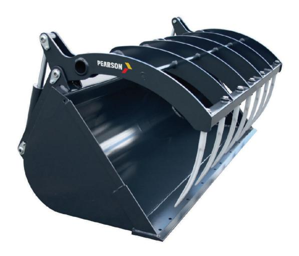
A reinforced version of the Telehandler Bucket which is bigger in size and sturdy in design. No need to change implements as this bucket is ideal for feeding and loading multiple products. Gain optimum wear life with a heavy duty 25mm thick x 200mm wide cutting edge, made from durable 450HB abrasion resistant steel. An easy clean design allows for efficiency and ease of use as well.
