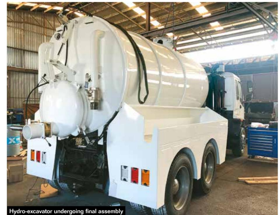
Hydro-excavator undergoing final assembly
