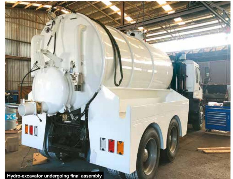
Hydro-excavator undergoing final assembly
