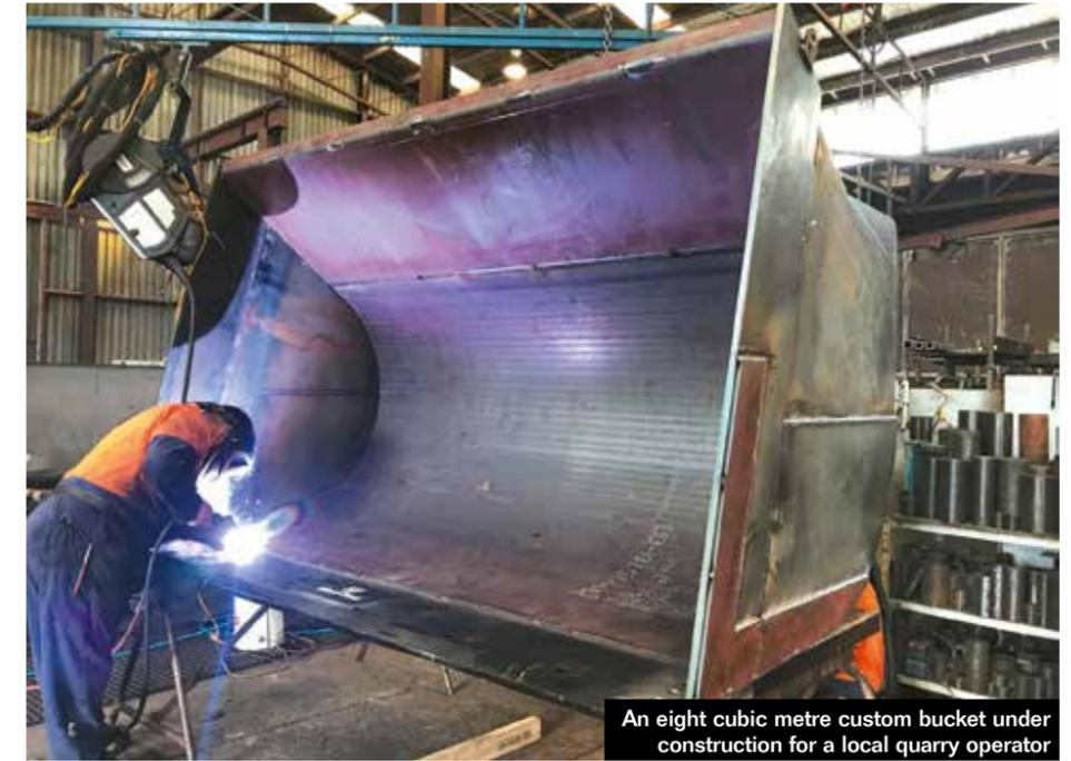
An eight cubic metre custom bucket under construction for a local quarry operator
