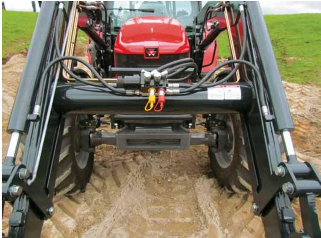
the loader both top and bottom for maximum strength. The mounting brackets are made from 20mm plates that are pressed and robotically drilled to ensure the best possible strength is achieved no matter what model tractor you have. All pin holes are fitted with grease-retaining replaceable bushes and all 35mm pins are machine cut and robotically welded to ensure a precise fit so there is no room for movement. All of Pearson Engineering's products are built
